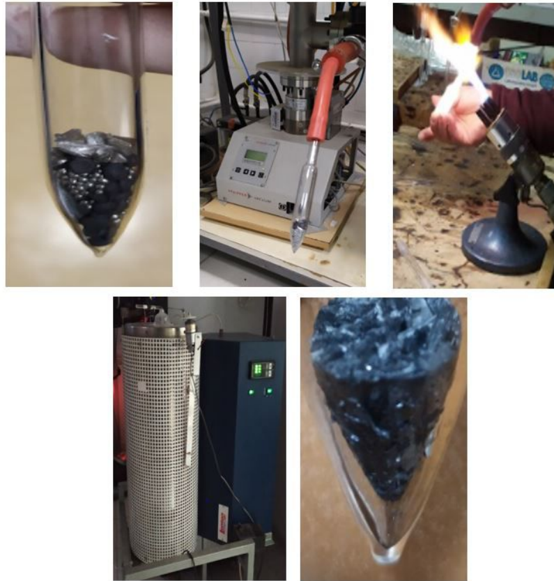
Figure 3.1: The sintering process of amorphous \text{SnSbSe}_2 ingot
